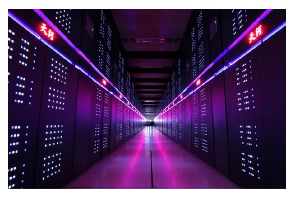
World's top supercomputer: Tihane-2 (China), 33.86 petaflops, 16000 nodes, 3,120,000 cores, 88 GB RAM at each node
